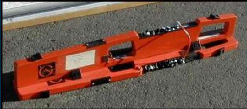
Figure 1. The Geonics EM38-DD conductivity meter.
